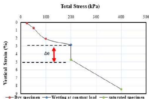
Figure 7. Collapse test results on the gypseous soil treated with 0.5% Nano silica
