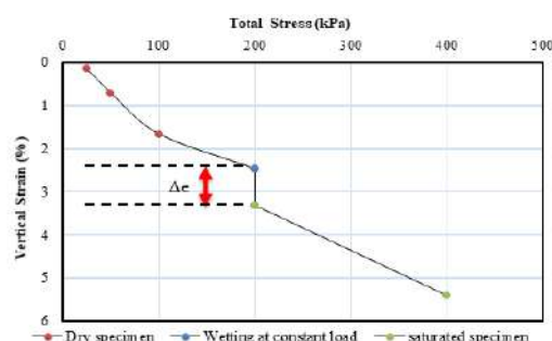
Figure 6. Collapse test results on the gypseous soil treated with 10% Nano clay
