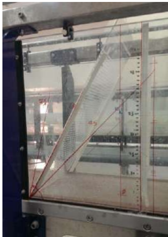
Figure 12. Selected angles of obstacle installation beyond 90°
