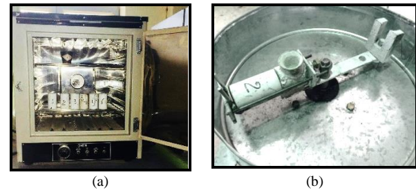
Figure 2. (a) The electric oven type ILE India for preheated the plaster molds; (b) The fabricated centrifugal rotor head plaster-mold cavity
