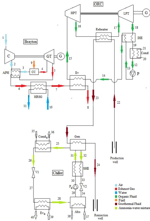
Figure 1. A schematic view of proposed triple generation system
