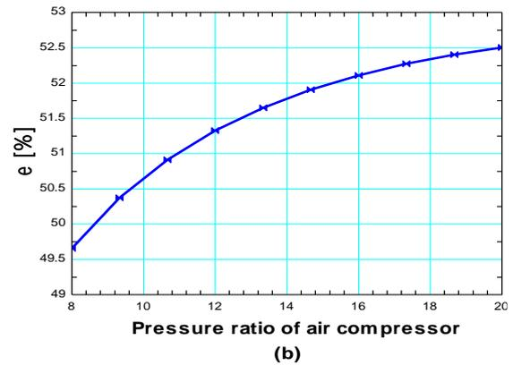
**Figure 2.** Compressor's pressure ratio effect on a) heating capacity of steam generator and refrigeration capacity of absorption chiller and b) exergy efficiency
