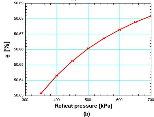
**Figure 3.** Reheating pressure effect on a) evaporator's refrigeration capacity and COP of absorption chiller cycle and b) exergy efficiency of system
