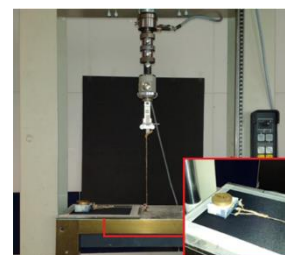
Figure 7. Testing equipment used for the friction between fabric and lining samples
