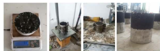
Figure 2. Manufacturing composite pavement specimens
