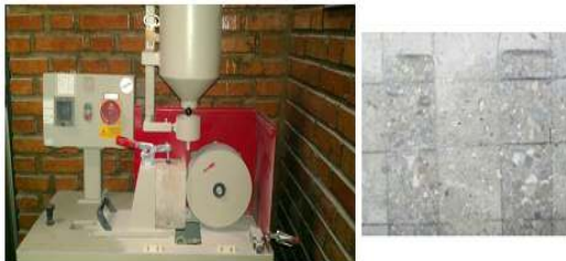
Figure 5. The test procedure of abrasion resistance according to EN 1338 and the grooved width of the specimens
