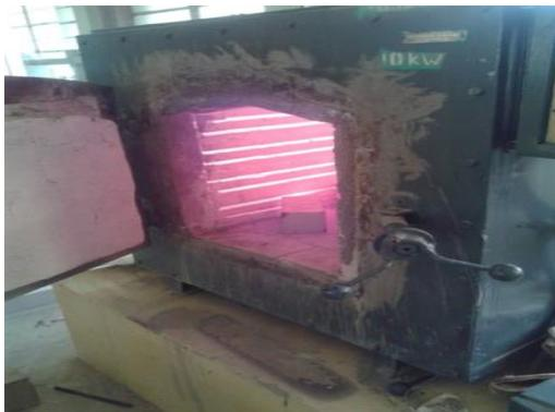
Figure 3. Heating the brick using furnace
