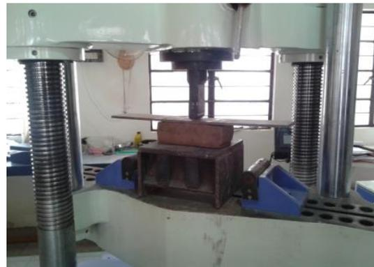
Figure 5. Testing of brick using 50T Universal Testing machine (UTM)
