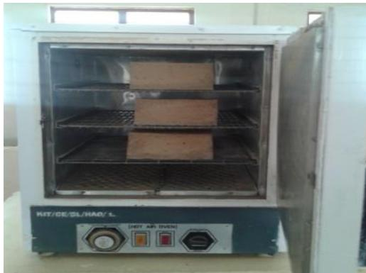
Figure 4. Heating the brick using Hot air Oven
