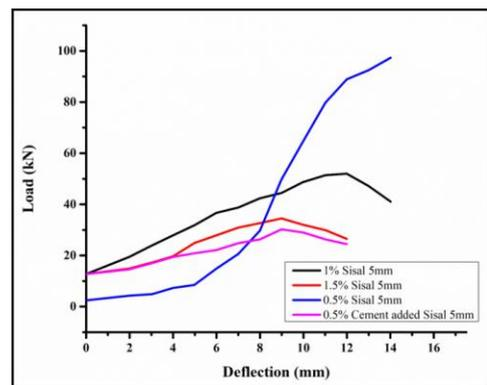
**Figure 9.** 5mm Sisal Fibre at 0.5, 1 and 1.5%
