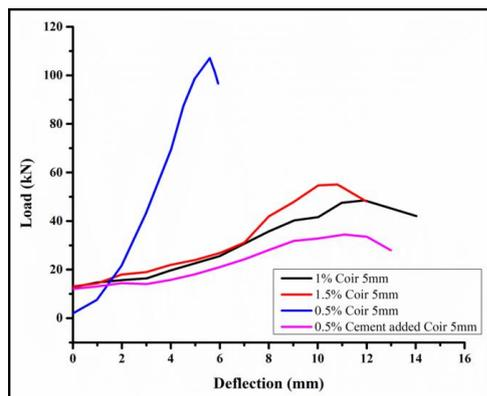
Figure 10. 5mm Coir Fibre at 0.5, 1 and 1.5%
