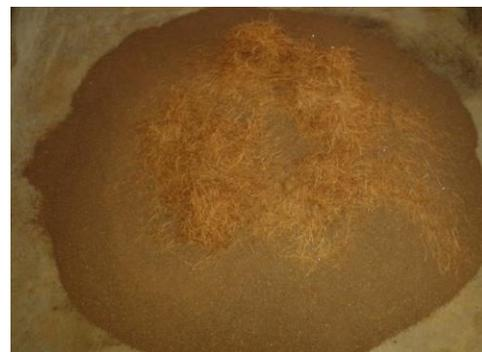
**Figure 1.** Mixing the fibre with clay soil
