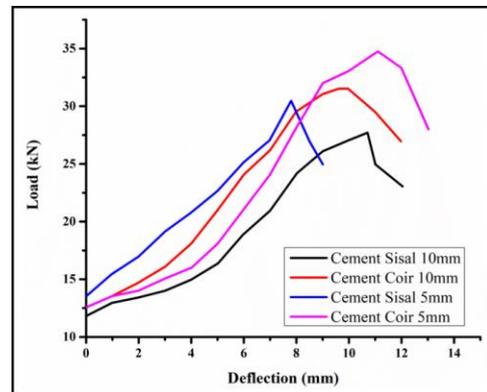
**Figure 8.** 10mm and 5mm Sisal , coir fibre with 5% of cement
