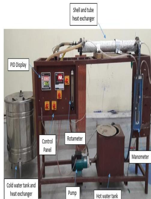
Figure 2. Photographic presentation of experimental setup.
