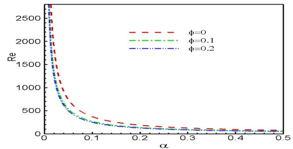
Figure 8. Critical relation between  $\alpha$  and  $Re$  for different values of  $\phi$  at  $Ha = 1$  obtained by HODA for  $d = 7$ .
