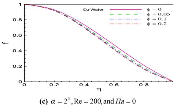
**Figure 4.** Effects of nanoparticle volume fraction on velocity profiles for Cu-Water.
