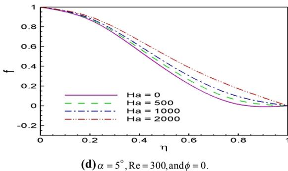
**Figure 3.** Velocity profiles in divergent channel with different values of  $Ha$  and  $Re$ .
