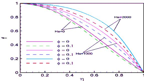
Figure 5. Velocity profiles for several values of Hartmann number and solid volume fraction at  $\alpha = 5^\circ, Re = 50$ .
