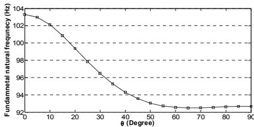
Figure 2. Effect of fiber orientation angle ( $\theta$ ) on fundamental natural frequency of stacking  $[\pm 45_{glass}/0_{carbon}/\theta_{glass}]$
