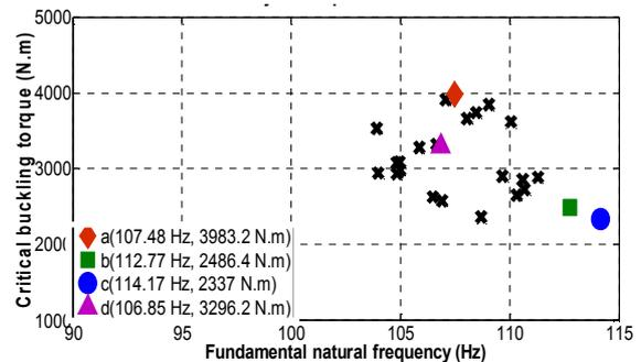
**Figure 8.** Critical buckling torque versus fundamental natural frequency in 3-objective optimization
