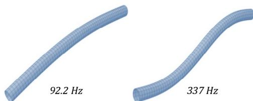
Figure 4. The first (left) and second (right) mode shapes of composite tube and their corresponding frequency values.
