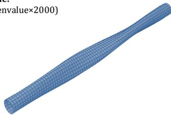
**Figure 7.** First torsional buckling mode and its corresponding eigenvalue and buckling torque
