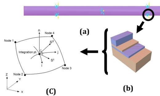
**Figure 1.** (a) Composite tube model in ABAQUS, with fiber orientation depicted on it (b) composite laminate configuration [90, +45, -45, 0] (c) S4R element geometry.
