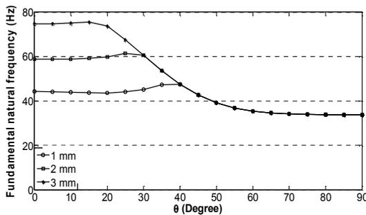
Figure 3. Effect of ply thickness on fundamental natural frequency.  $\theta$  is changing between 0 to 90 degree in  $[\pm \theta_{glass}]_2$  stacking. Legend shows the total thickness of composite tube
