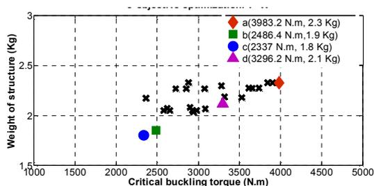
**Figure 10.** Total weight of structure versus critical buckling torque in 3-objective optimization
