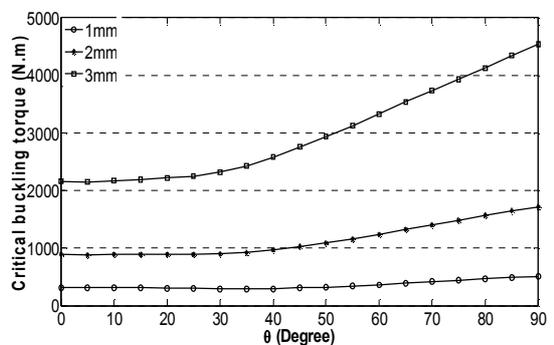
Figure 6. Effect of ply thickness on critical buckling torque.  $\theta$  is changing between 0 to 90 degree in  $[\pm \theta_{glass}]_2$  stacking. Legend shows the total thickness of composite tube
