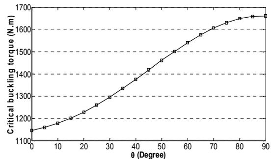
Figure 5. Effect of fiber orientation angle ( $\theta$ ) on critical buckling torque of stacking  $[\pm 45_{glass}/0_{carbon}/\theta_{glass}]$
