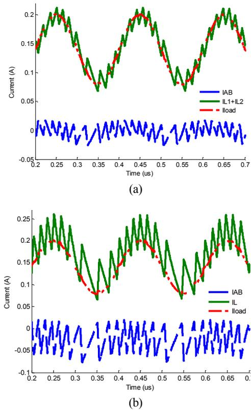
**Figure 15.** Time domain waveforms of class D, class AB and load resistance output current a) two-phase b) single phase
