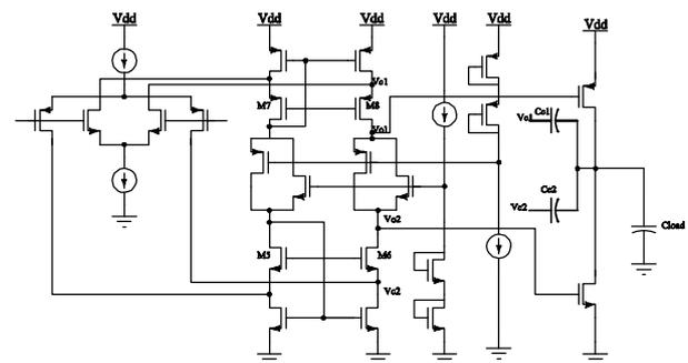
Figure 3. Class AB power amplifier architecture
