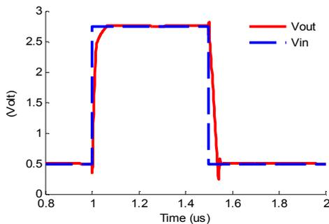
Figure 5. Class AB PA tracking a 10 MHz (0.5-2.7 V) square wave
