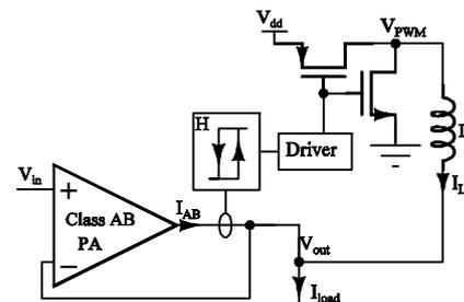
Figure 2. Block diagram of HSEM
