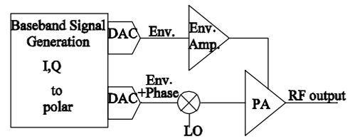
Figure 1. Block diagram of envelope tracking power amplifier
