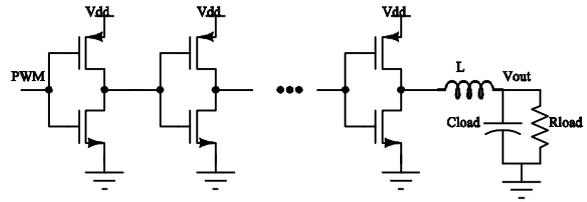
Figure 14. Class D power amplifier with driver stages
