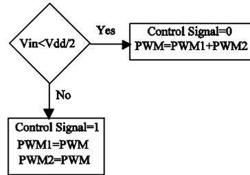
Figure 13. Flowchart of reconfigurable IL sharing control block operation principle
