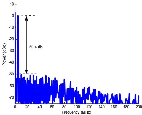
**Figure 17.** Power spectrum of the output voltage of two-phase modulator for 5 MHz signal at Pout=27.4 dBm
