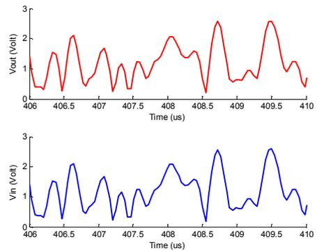
**Figure 20.** Simulated 5 MHz WiMAX time-domain waveforms of the proposed digital supply modulator.
