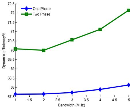
**Figure 19.** Simulated dynamic efficiency of the envelope modulator versus input signal bandwidth at Pout=27.4 dBm
