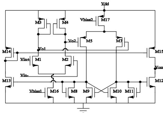
Figure 10. Voltage hysteretic circuit used for block H1
