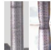
Figure 2. Two sequences of a tensile test
