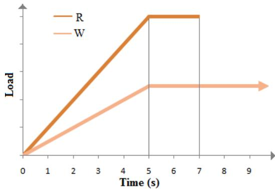
Figure 3. Applied loads for column removal analysis
