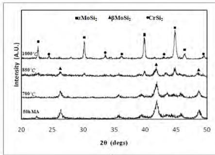
**Fig. 5.** XRD patterns of the annealed powders that 50 h milled with 0.4 Cr at the cup speed of 640 rpm.
