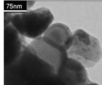
**Fig. 6.** Bright field image of the 50 h milled powder with 0.1 at.% Cr.
