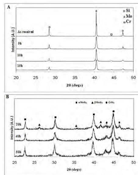
**Fig. 1.** XRD patterns of the as milled powders with 0.1 at.% Cr at the cup speed of 640 rpm.
