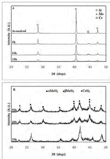
**Fig. 2.** XRD patterns of the as milled powders with 0.25 at.% Cr at the cup speed of 640 rpm.
