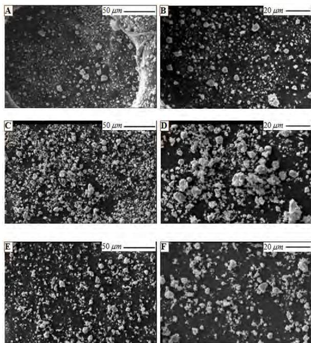
**Fig. 7.** SEM images of the 50 h milled powders at the cup speed of 640 rpm with different Cr content: A) 0.1at.%, B) 0.1at.% at higher magnification (HM), C) 0.25at.%, D) 0.25at.% (HM), E) 0.4at.% and F) 0.4at.% (HM)
