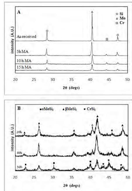
**Fig. 3.** XRD pattern of the as milled powders with 0.4 at.% Cr at the cup speed of 640 rpm.
