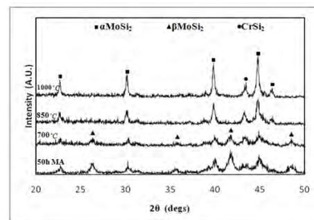
**Fig. 4.** Effect of the annealing on the structure of the 50 h milled powder with 0.25 at.% Cr at the cup speed of 640 rpm.
