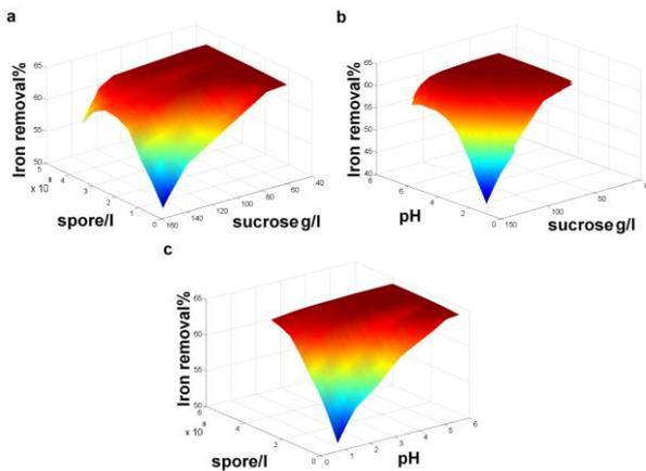
**Figure 4.** 3D plot of Iron removal as function of initial pH, sucrose and spore concentration.
