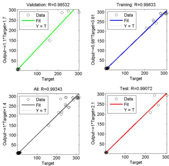
**Figure 3.** Correlation between the predicted value of Iron concentration with experimental value for validation, test and train data
