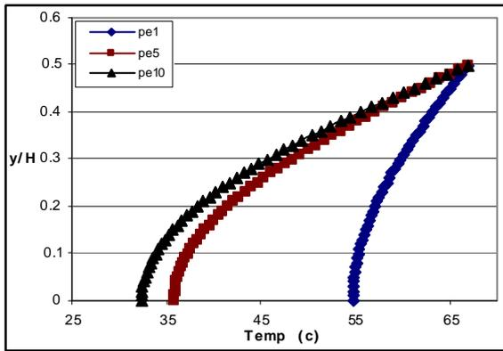
**Figure 11.** Peclet number effects on temperature distribution which shows temperature profile at different Peclet number and constant dimensionless length.  $\xi = 0.3$
