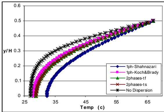
**Figure 7.** Comparison of temperature distributions for different correlations of thermal dispersion.  $Pe = 10$  ,  $\xi = 0.3$
