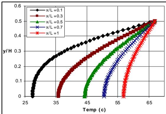
**Figure 3.** Comparison of temperature distribution in various dimensionless length of channel at constant Peclet number.  $Pe = 5$
