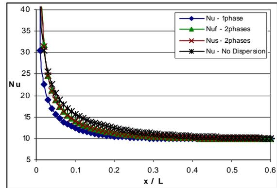
**Figure 9.** Thermal dispersion effects on local Nusselt number in different models at constant Peclet number.  $Pe = 5$
