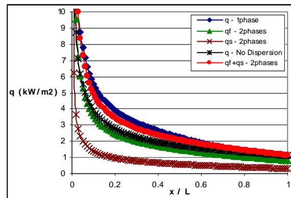
**Figure 10.** Thermal dispersion effects on heat flux in different models at constant Peclet number.  $Pe = 5$
