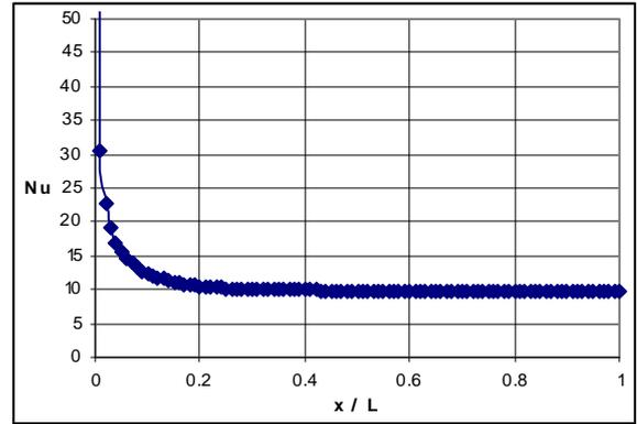
**Figure 5.** Local Nusselt number to dimensionless length of channel at constant Peclet number.  $Pe = 5$
