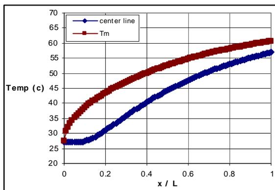
**Figure 4.** Center line and cross section mean temperature to dimensionless length of channel at constant Peclet number.  $Pe = 5$
