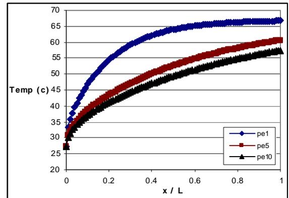
**Figure 13.** Peclet number effects on cross section mean temperature to dimensionless length of channel which shows cross section mean temperature at different Peclet number.
