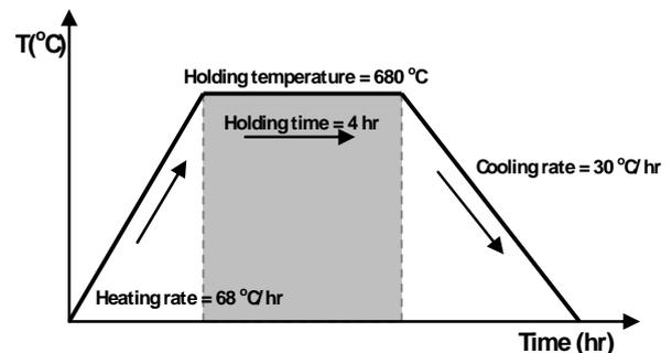
Figure 8. The tempering heat treatment procedure applied in failed section of rotor.
