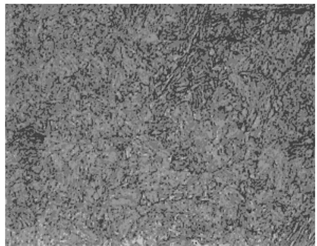
**Figure 4.** The micro structural variations on embrittled zone of journal surface (Etchant: 2 % Nital, 100 X).
