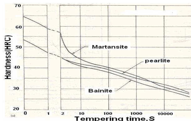
**Figure1.** The effect of microstructure on hardness during tempering [8].
