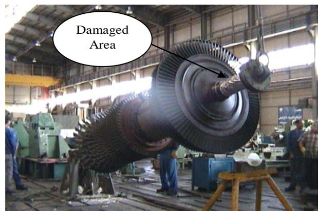
Figure 2. A general view of damaged rotor in journal position.
