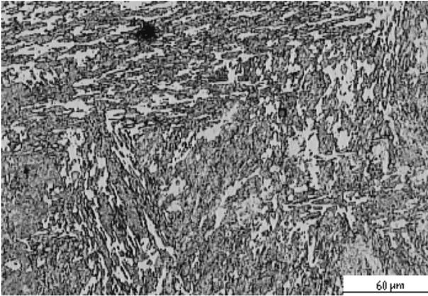
**Figure 5.** The safe or original structure of rotor steel (enchant 2 % Nital) [7,11].
