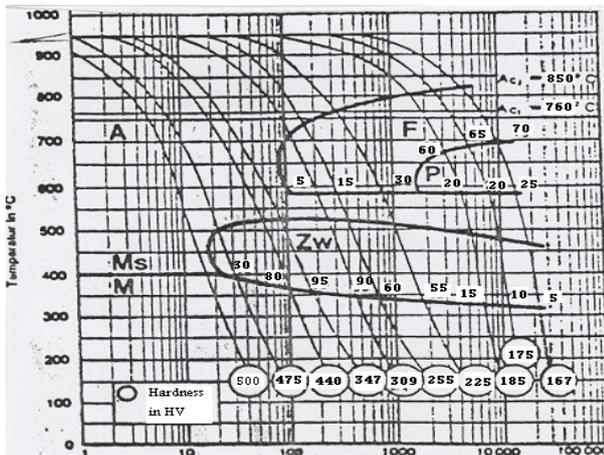
**Figure 6.** Continuous-cooling-transformation diagram (C.C.T) for A470/CrMoV steel [11].
