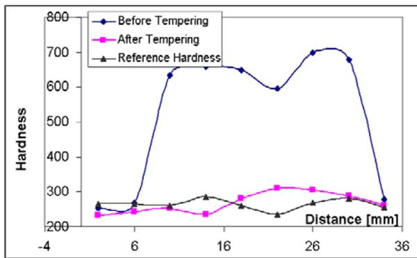
**Figure 10.** The results of tempering heat treatment applied in failed section of rotor with comparison to before and after tempering.
