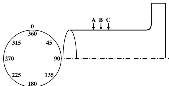
**Figure 3.** Hardness test locations in the peripheral and longitudinal directions of shaft with dimensions D = 204 mm, L = 160 mm.
