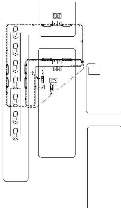
Figure 11. Recommended Layout of Transportation System for Door Cell.
