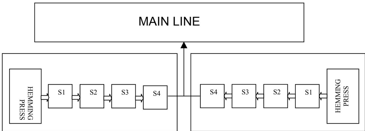
Figure 10. Recommended Layout of Door Cell.
