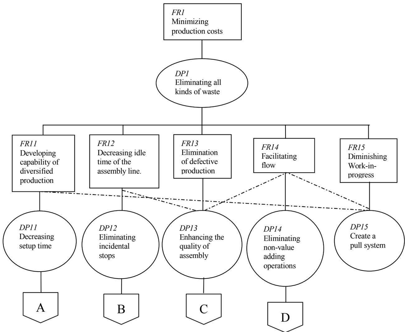
Figure 2. Second Level of the Developed Structure.
