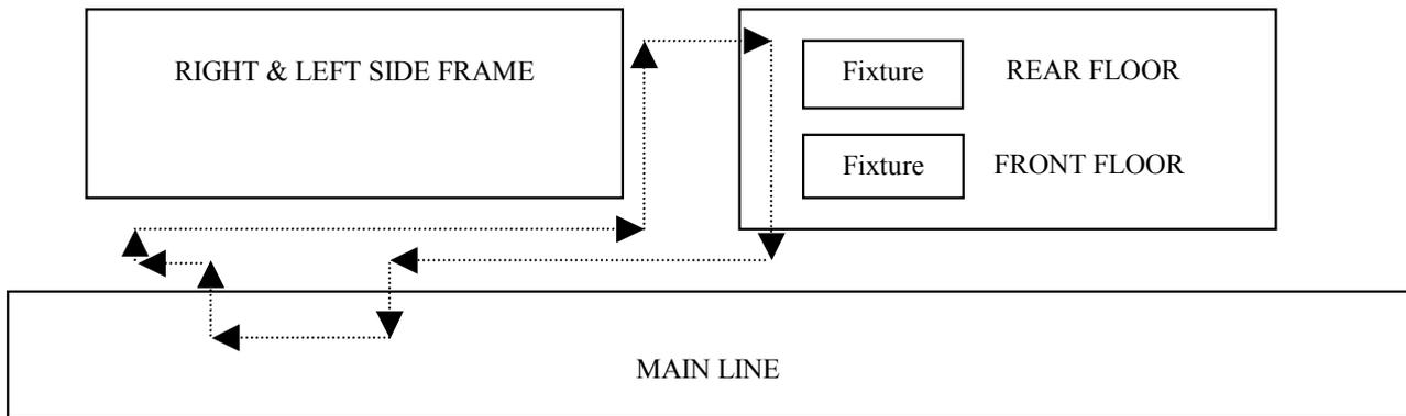
Figure 14. Recommended Layout of Transportation System for Underbody Cell.
