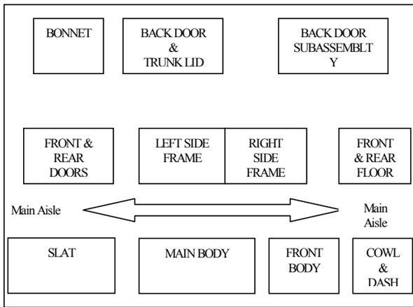
Figure 8. General Layout of the Body Assembly Line.
