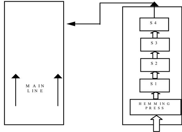
Figure 9. Existing Layout of Door Cell.
