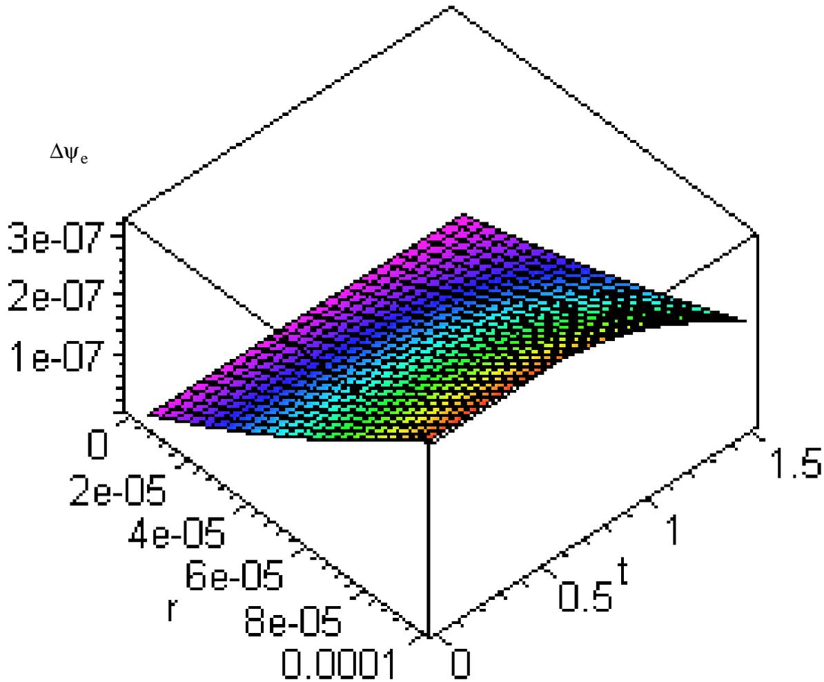
Figure 7. Change in availability with respect to initial state versus radius and contact angle.
