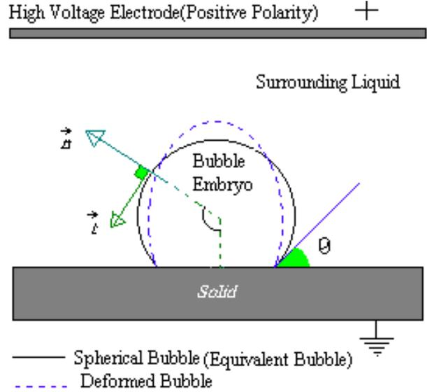
**Figure 4.** Attached bubble embryo on solid surface as a heterogeneous nucleation.
