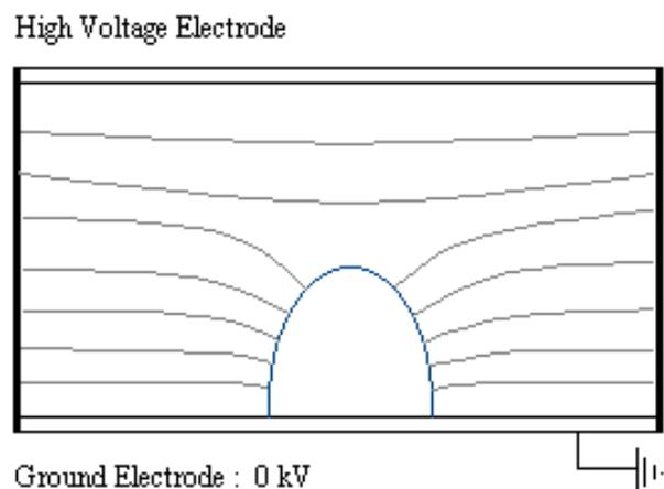
**Figure 2.** Equipotential lines around an attached bubble in a uniform electric field.
