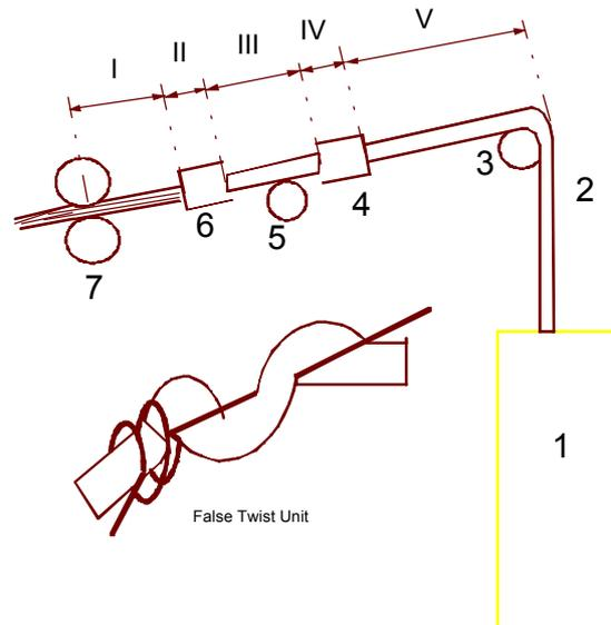
Figure 2. Schematic diagram of a passive false-twist simulator device with two false-twist units.
