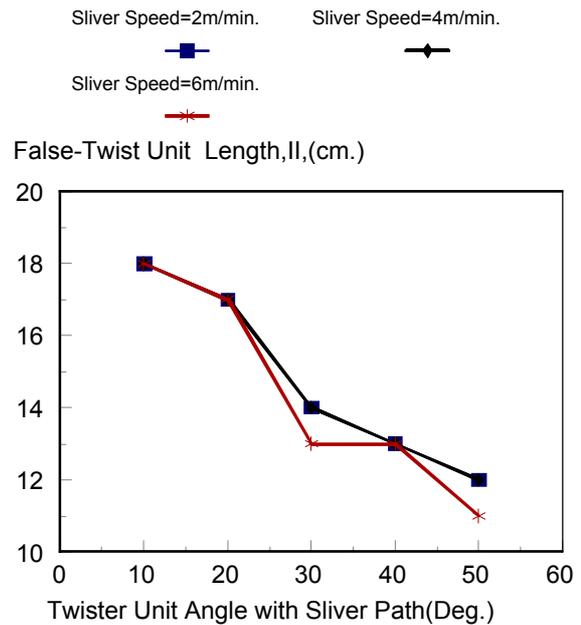
**Figure 12.** Effect of sliver speed on false-twist length (II). Wire diameter = 2mm., sliver speed = 2m/min. and No. of sliver turns around the wire = 1.
