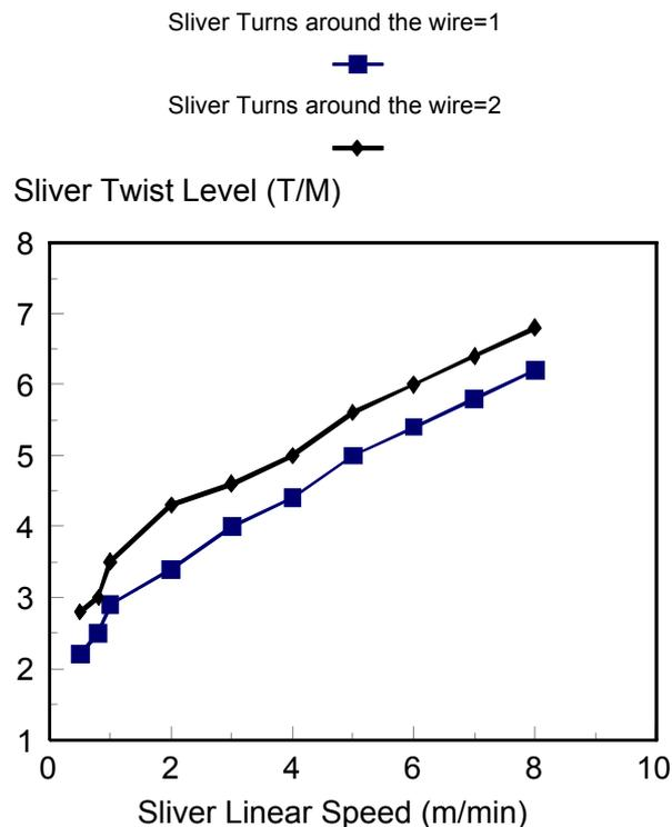
**Figure 6.** Effect of sliver speed on sliver twist. Wire diameter = 2mm, sliver count = 2.5 Ktex and wire angle = 30 (Deg.).
