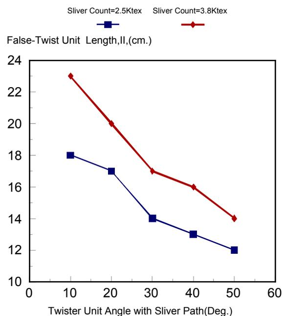
**Figure 13.** Effect of sliver count on false-twist length (II). Wire diameter = 2mm, sliver speed = 2m/min. and No. of sliver turns around the wire = 1.
