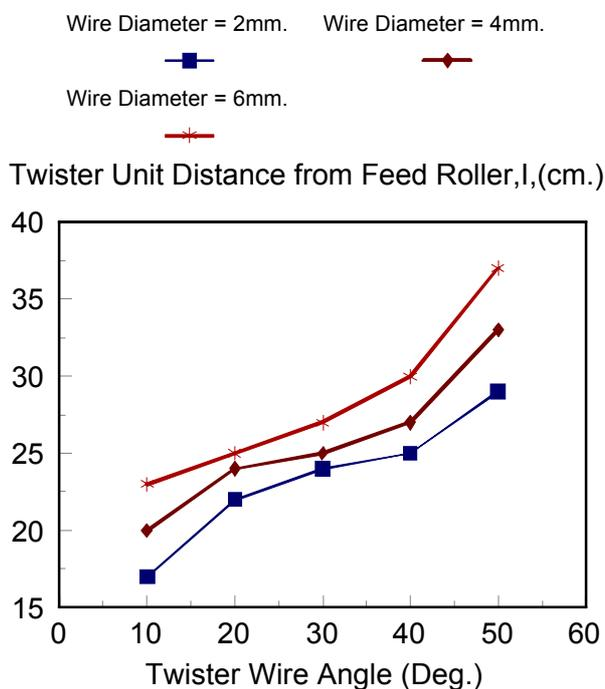
**Figure 7.** Effect of wire diameter and angle on twister unit distance (I) from feed roller. No. of sliver turns around the wire=1, sliver count=2.5Ktex, sliver speed=2m/min.
