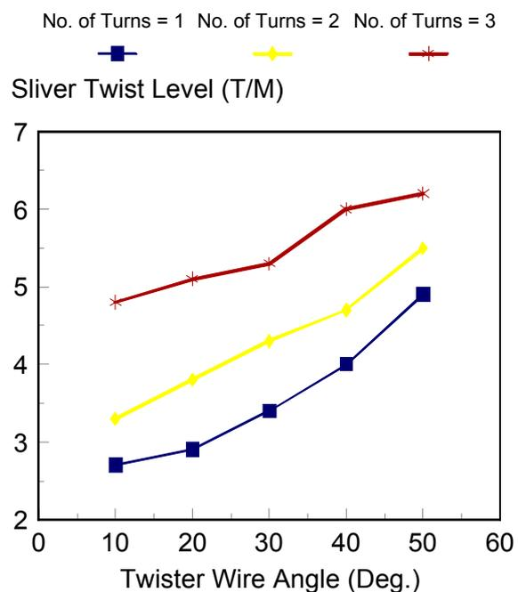
Figure 4. Effect of No. of turns of the sliver around the twister wire on sliver twist level. Sliver count = 2.5 Ktex, sliver speed = 2 m/min, twister wire diameter = 2 mm.
