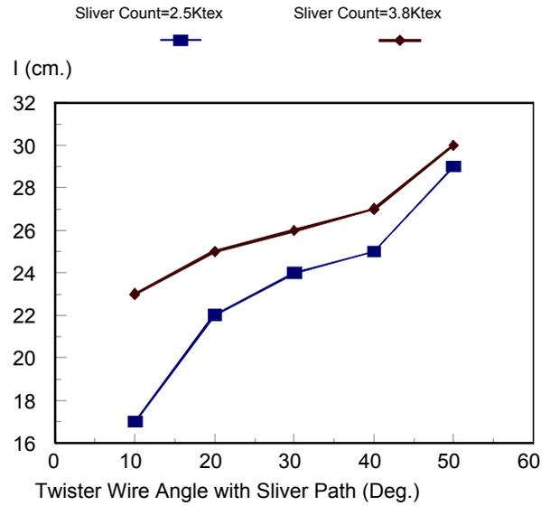
**Figure 10.** Effect of sliver count on twister unit distance from feed roller (I). Wire diameter = 2mm., sliver speed = 2m/min. and No. of sliver turns around the wire = 1.
