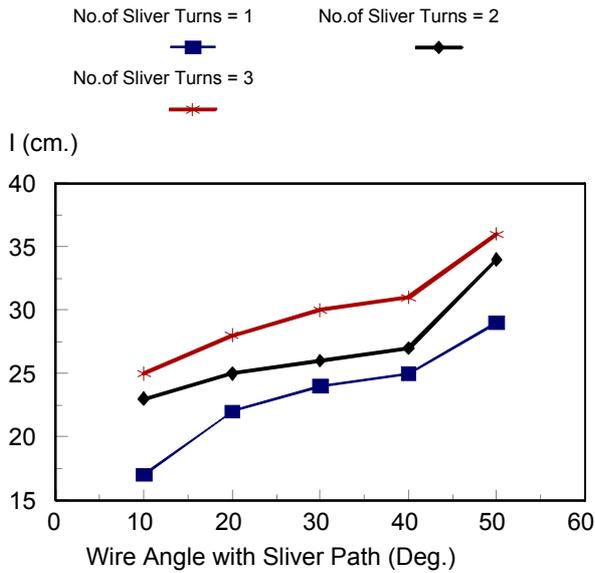
**Figure 8.** Effect of No. of Sliver Turns around the Twister Wire on Twister Unit Distance from Feed Roller (I). Sliver Count = 2.5 Ktex, Sliver Speed = 2m/min and Wire Diameter = 2 mm.
