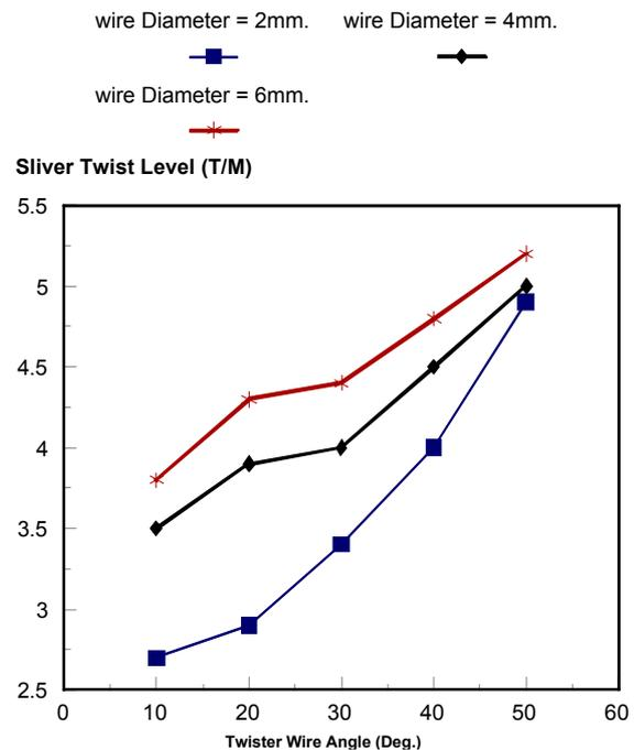
Figure 3. Effect of the twister wire diameter and angle on sliver twist level.No. of sliver turns around the twister wire = 1, Sliver count = 2.5 Ktex, sliver speed = 2 m/min.
