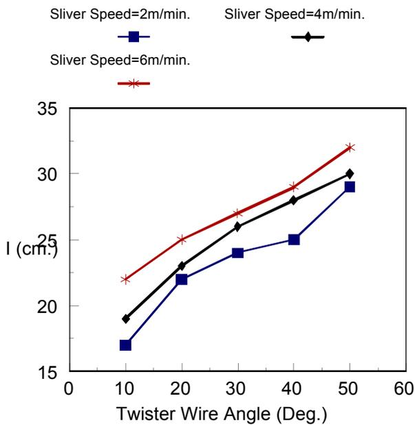
**Figure 9.** Effect of sliver speed on twister unit distance from feed roller (I). Wire diameter = 2 mm., sliver count = 2.5 Ktex and No. of sliver turns around the twister wire = 1.
