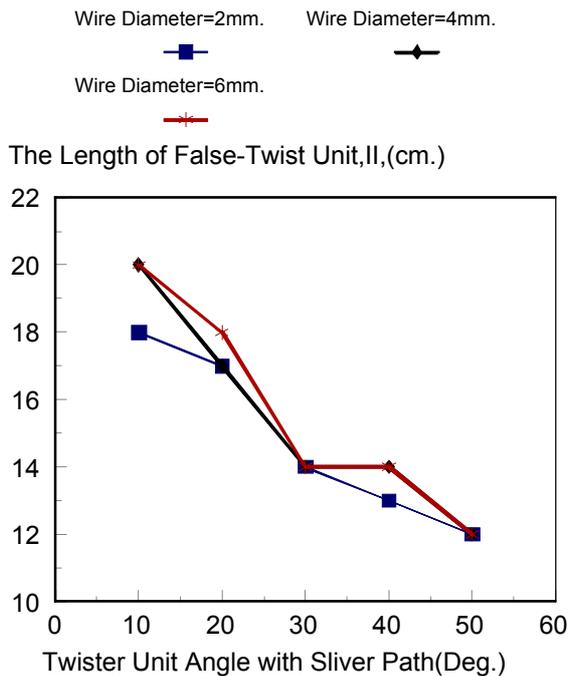
**Figure 11.** The effect of wire diameter and twister unit angle with sliver path on false-twist length (II). Wire diameter = 2mm., sliver speed = 2 m/min. and No. of sliver turns around the wire = 1.
