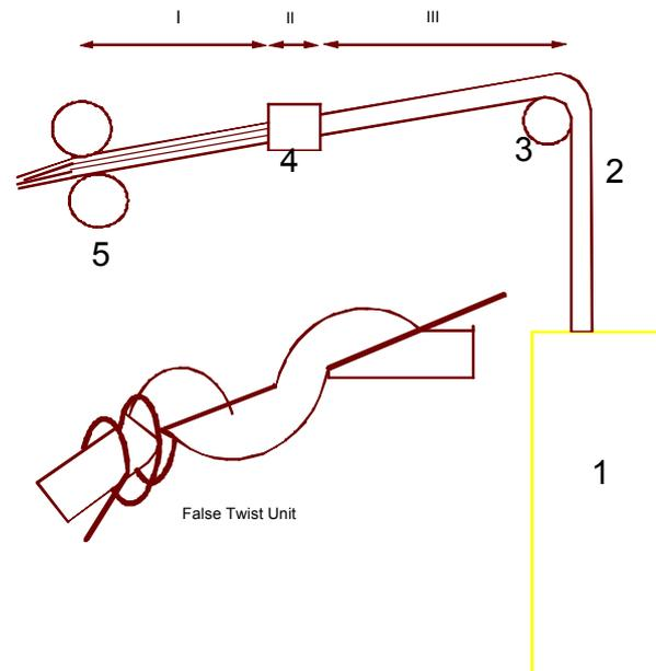
**Figure 1.** Schematic diagram of a passive false-twist simulator device with one false-twist unit.
