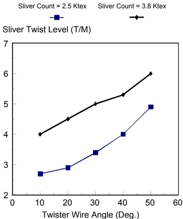
**Figure 5.** Effect of sliver count on sliver twist level. No. of sliver turns around the wire =1, sliver speed = 2 m/min and twister wire diameter = 2 mm.
