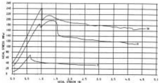
**Figure 3.** Stress–strain plots for sandstone specimens with natural joints, joint angle = 45°, confining pressures = 5, 10, 15 and 30 MPa.
