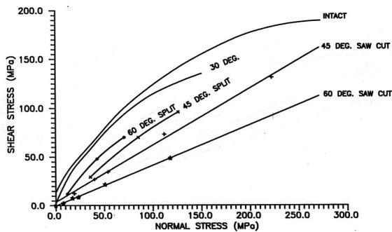
**Figure 6.** Mohr envelopes for intact and jointed (saw cut and split) sandstone specimens (type I).
