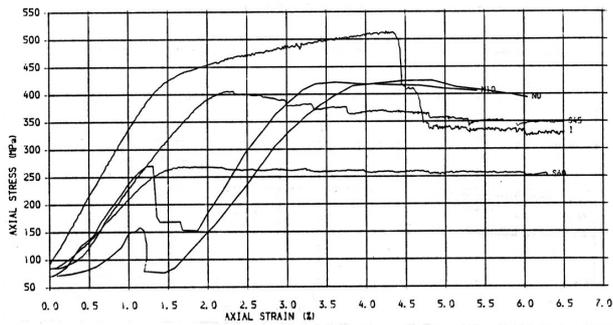
**Figure 5.** Stress–strain plots for intact and jointed sandstone specimens, saw cut with 45 and 60°, and shear-surface joints (at 0 and 10 MPa), confining pressure 70 MPa.
