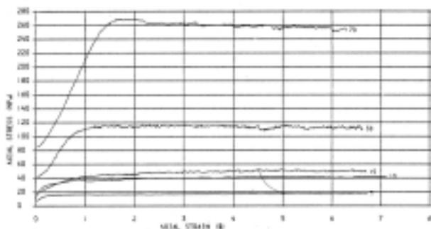
**Figure 2.** Stress–strain plots for sandstone specimens with saw cut joints, joint angle = 60°, confining pressures = 5, 10, 15, 30 and 70 MPa.
