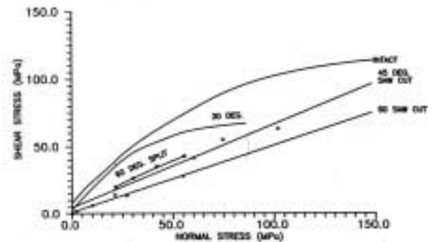
**Figure 7.** Mohr envelopes for intact and jointed (saw cut and split) sandstone specimens (type II).
