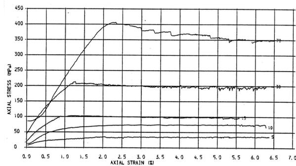
**Figure 1.** Stress–strain plots for sandstone with saw cut joints, joint angle = 45°, confining pressures = 5, 10, 15, 30 and 70 MPa.
