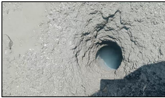
Figure 7. Post-blasting effect on borehole
