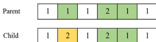
Figure 12. The mutation operator in the HNSGAI-PSO algorithm
