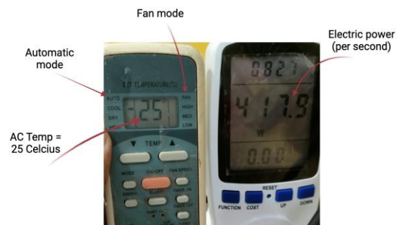
Figure 3. Manual Measurement Process of Electric Power at AC Temperature = 25°C
