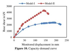
mm at 2512.56 kN base shear in Model-I and a maximum inelastic displacement of 329.14 mm at 6612.51 kN base shear. This result says that the capacity of Model-II (Figure 11) is more as it experiences more inelastic deformations by absorbing more amount of base shear compared to Model-I.
