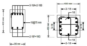
Figure 3. Designed section details of beams and columns in Model-I
