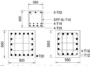
Figure 4. Designed section details of beams, columns in Model-II
