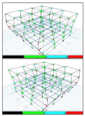
Figure 6. Maximum target displacement and hinge response at that point
