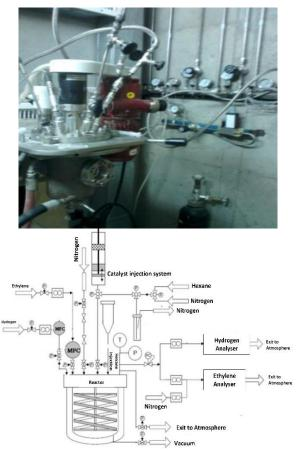
Figure 1. The experimental set up for copolymerization of ethylene/1-butylene and its scheme
