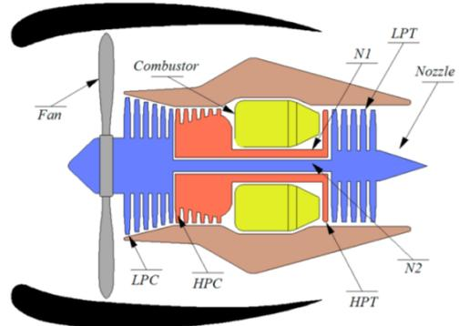
**Figure 1.** Simplified diagram of the gas turbine engine [22]
