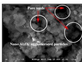
**Figure 1a.** SEM image of the Nano- $\text{Al}_2\text{O}_3$
