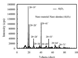
**Figure 1b.** XRD image of the Nano- $\text{Al}_2\text{O}_3$
