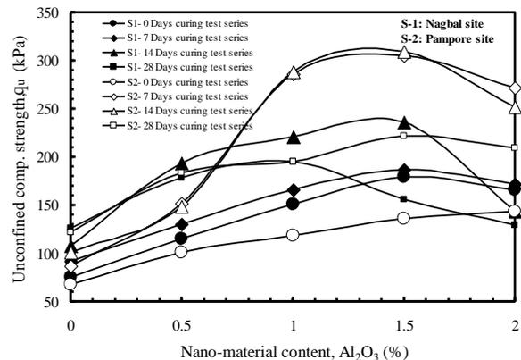
Figure 4. Variation in UCS for nano-material (Al<sub>2</sub>O<sub>3</sub>) stabilized soil samples
