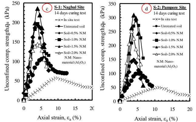
Figure 3. Effect of nano-Al<sub>2</sub>O<sub>3</sub> content on stress-strain behaviour of soil collected from site-1 (a & c) & site-2 (b & d) for different curing periods (0 and 14 days)
