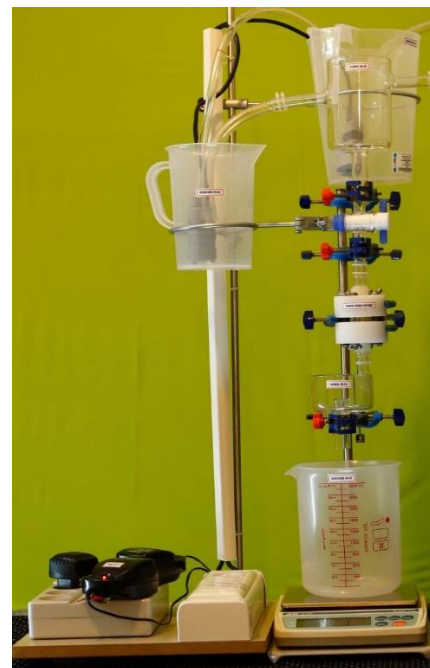
Figure 3. The 3D model of designed constant head permeability test setup, (1) Fluid storage tank, (2) Upper reservoir, (3) Valve, (4) Fixture, (5) Lower reservoir, (6) Collector, (7) Electronic scale, (8) Overflow fluid tank.
