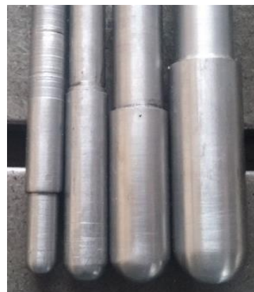
Figure 8. Cylindrical tools with diameters of 5, 8, 12 and 16 mm
