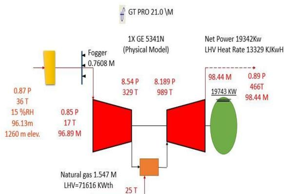
Figure 7. Output results of simulation with a fog system
