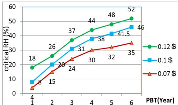
**Figure 10.** Critical RH variation with electricity price in Iran and PBT
