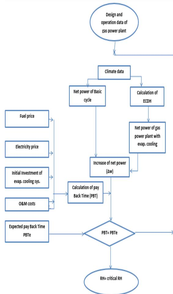
Figure 8. Flow chart for finding critical RH
