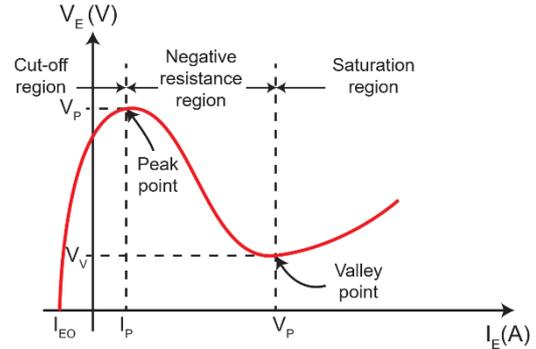
**Figure 2.** Static emitter current-voltage characteristic for a Unipolar Junction Transistor
