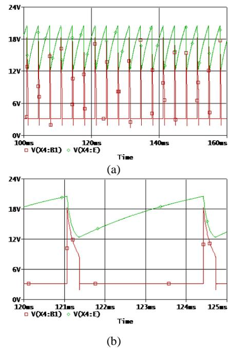
Figure 5. Neuron emulator waveforms. (a) The voltages of the capacitor and the resistor R1 vs. time (b) Zoomed the voltages of the capacitor and the resistor R1 vs. time
