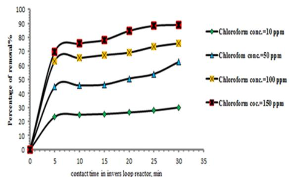
**Figure 5.** Impact of contact time on the percentage of removal of  $\text{CHCl}_3$  with various initial concentrations of  $\text{CHCl}_3$  during the occurring of stripping, oxidation, and adsorption processes in reverse fluidizing reactor
