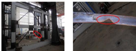
Figure 2. Concrete frame strengthened by steel brace and its fracture mode [9]
