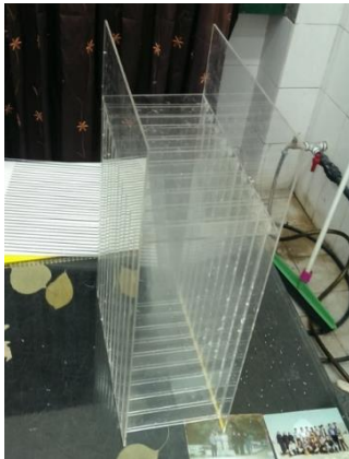
Figure 15. Example of obstacle with dimension for testing impact of obstacle thickness
