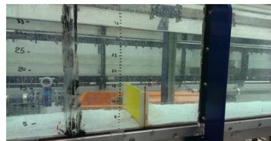
Figure 18. View of deposited material with second layer of obstacle
