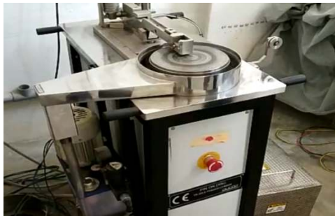
Figure 5. Pin on Disc experimental setup
