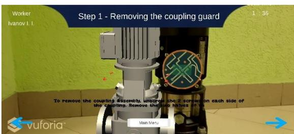
Figure 8. Unscrew two screws of coupling guard
