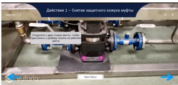
Figure 6. Removing pump from laboratory unit
