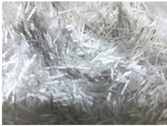
Figure 3. Glass fiber used in concrete specimens
