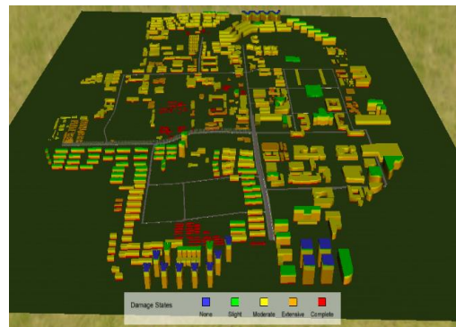
Figure 6. The high-fidelity building seismic damage of the campus
