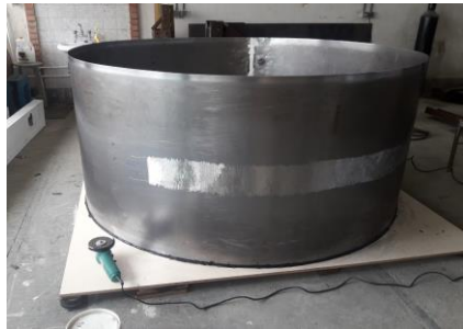
Figure 5. Milling the position of the CFRP ring
