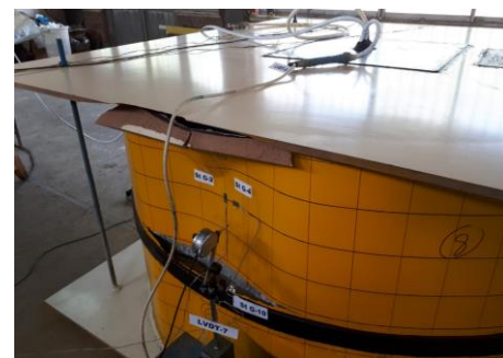
Figure 7. failure after ultimate buckling
