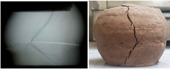
Figure 11. the reinforced sample with one layer of geocomposites
