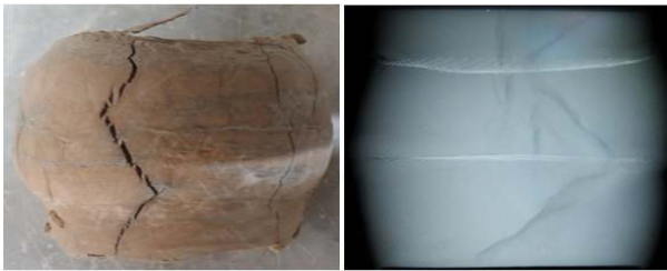
Figure 12. the reinforced sample with two layers of geocomposites
