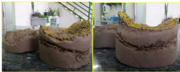
Figure 13. Behavior of Geogrid in different stages
