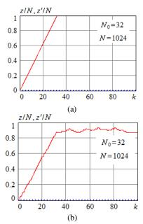
**Figure 7.** The normalized responses of the signal extraction channel and the interference estimate channel in the absence of interferences
