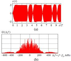
Figure 1. PSK signal and its spectrum
