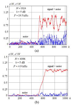
**Figure 9.** The normalized responses of the signal extraction channel and the interference estimate channel in the presence and in the absence of the signal
