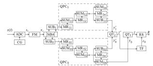
Figure 2. Digital PSK signal detector
