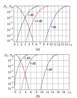
**Figure 12.** The false alarm and the missing probabilities under N = 1024 and N = 8192
