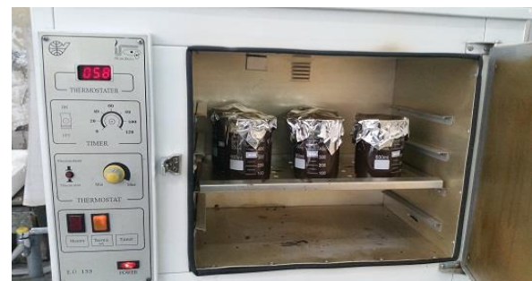
Figure 2. Tensile sample plunging in drilling mud sample and in down hole temperature of the oven
