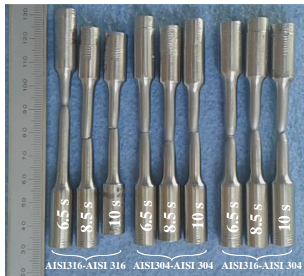
Figure 12. Macro-graphic of tensile test pieces
