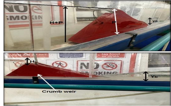
Figure 5. Flow over crump weir in condition of two open holes
