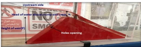
Figure 4. Flow over crump weir model
