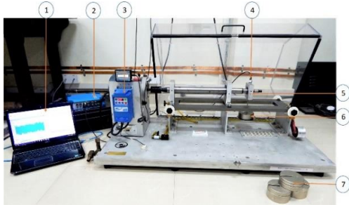
Figure 2. An Experimental Test Rig The labels are 1. Laptop; 2. Data acquisition system; 3. Variable frequency drive; 4. Uniaxial Accelerometer; 5. Specimen bearing with housing; 6. Radial Load; 7. Dead weights
