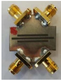
Figure 7. The photo of the fabricated coupler
