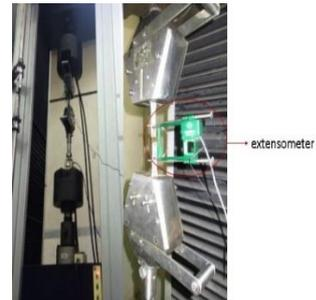
Figure 7. Tensile test machine and extensometer
