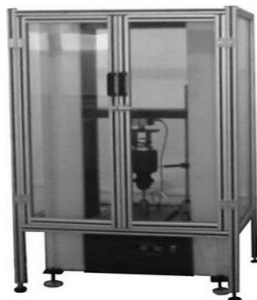
Figure 4. The stiffness characteristics testing of the air spring
