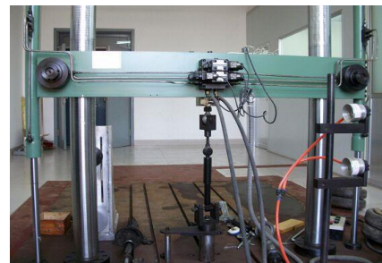
Figure 2. The damping characteristics test of the shock absorber
