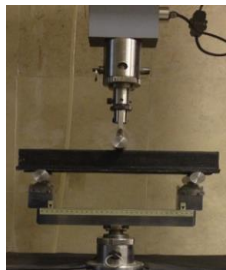
Figure 2. Three point bending test, the specimen and loading situations
