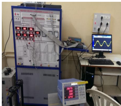
Figure 9. Experimental set up of 7-level DCMLI
